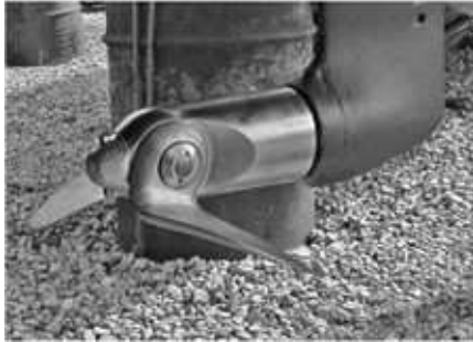
FIGURE 9-16. Top: What an Autoprop looks like in practice. Bottom: The way the blades are weighted causes one to hang down when under sail, creating a little more resistance than a feathering propeller. (Courtesy Brunton's Propellers)
