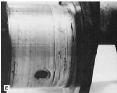
FIGURES 7-35A to 7-35E. Heat distortion (A)—discard. Corrosion of crankshaft journal (B)—discard. Heat distortion, plus material from the bearing shell is adhering to the journal (C)—discard. Cracked crankshaft (D)—discard. Smearing of bearing shell around the crankshaft (E)—discard. (Courtesy Caterpillar)
