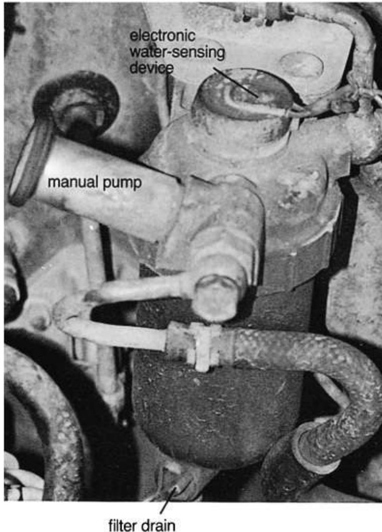
FIGURE 4-40. A manual fuel pump mounted on a fuel filter.
