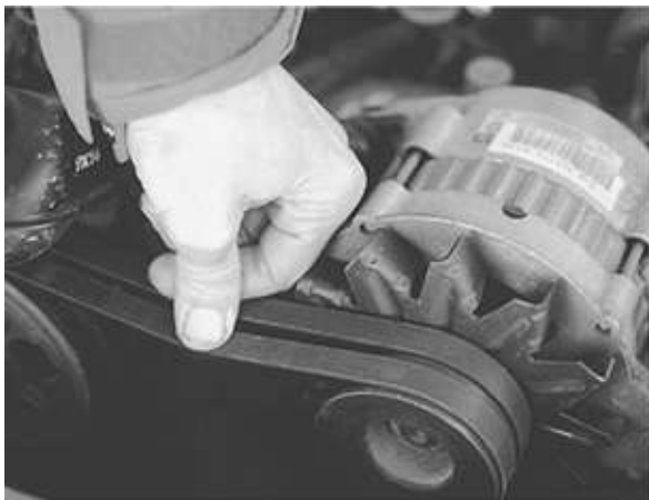
FIGURE 5-14. Checking belt tension.
