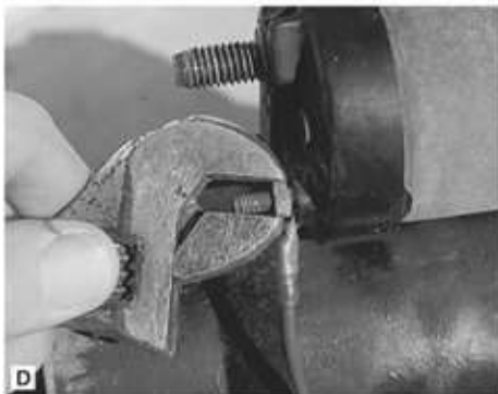
FIGURES 4-14A to 4-14K. Disassembling a preengaged starter's solenoid. First, identify the main components (A). Remove the battery cable (B). Disconnect the solenoid from the starter motor (C). Disconnect the cable to the ignition switch (D). Take the cover bolts off the solenoid (E and F). Bend the starter motor strap out of the way so the solenoid cover can be pulled off (G). Remove the solenoid cover (H); there is a spring in here that may fall out. A view of the contactor plate, showing the burned contactor (I). Note the severe pitting on the surfaces of the contactor (the circular disc) and the points (J). Sometimes the contactor can be flipped over to reveal an unused surface, and as in this case, the points can be rotated in their housing to bring a new surface into action (K). Otherwise, they can be filed and sanded smooth.
