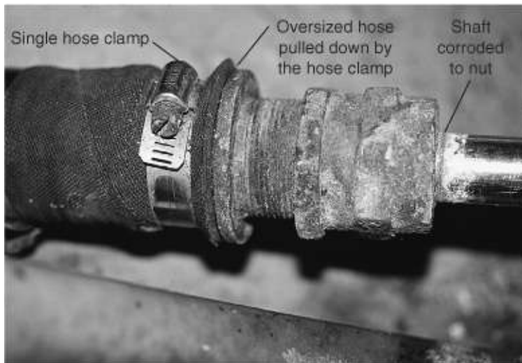
FIGURE 9-28. A stuffing box with single hose clamps in which the screws are 400-series stainless steel that is corroding. Meantime, the packing nut has corroded to the shaft. One way or another, when the engine is next put in gear, something is likely to tear loose, allowing large amounts of water to enter the boat!
