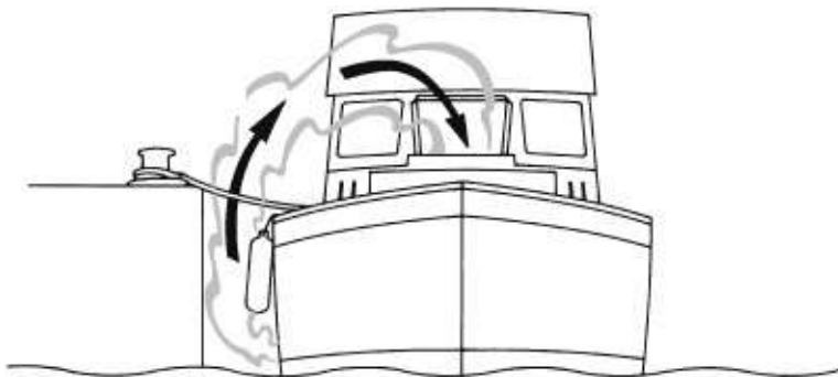
FIGURE A-1. Running an engine alongside a dock can put carbon monoxide into the boat. (Jim Sollers)
