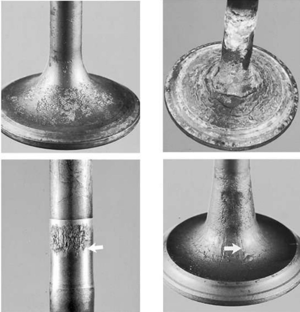
FIGURE 7-18. Valve failure. Top left and right: Corrosion from moisture and acids. Bottom right: Stress cracks caused by high temperature. Bottom left: Metal-to-metal transfer (galling) from a valve stem sticking in its guide. (Courtesy Caterpillar)
