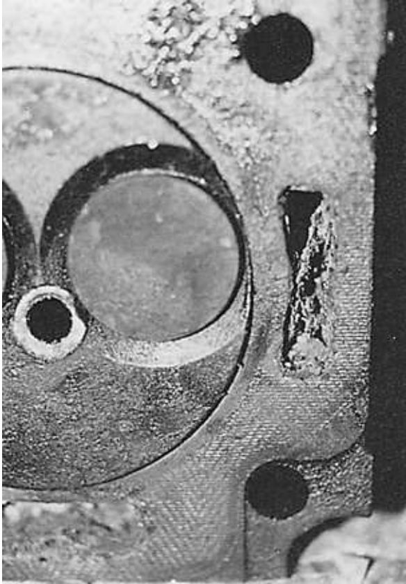
FIGURE 2-29. Corrosion in a raw-water-cooled cylinder head. Note the scale partially plugging the water passage on the right-hand side.
