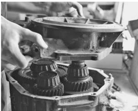
FIGURE 8-9. Removing the end cover from a larger two-shaft transmission. It would have been a good idea to clean the exterior before working on it! Note the
