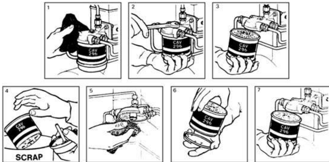
FIGURE 3-22. Changing a filter with a replaceable element. 1. Clean all external dirt from the unit before you service the filter. Unscrew the thumbscrew in the base and drain the accumulated water and sludge. 2. Unscrew the center bolt while you hold the base to prevent it from rotating. 3. Release the filter element complete with the base by pulling the element downward while turning it slightly so that it comes free from the internal O-ring. 4. Detach and discard the element. Detach and inspect the lower sealing ring for damage. Replace a defective O-ring. 5. Clean out the sedimenter base. Complete the cleaning by rinsing with clean diesel fuel. Clean the unit head and inspect both the upper sealing ring and the O-ring for damage. Replace any defective sealing rings. 6. New sealing rings are available from filter suppliers. 7. Check that the upper sealing ring and
