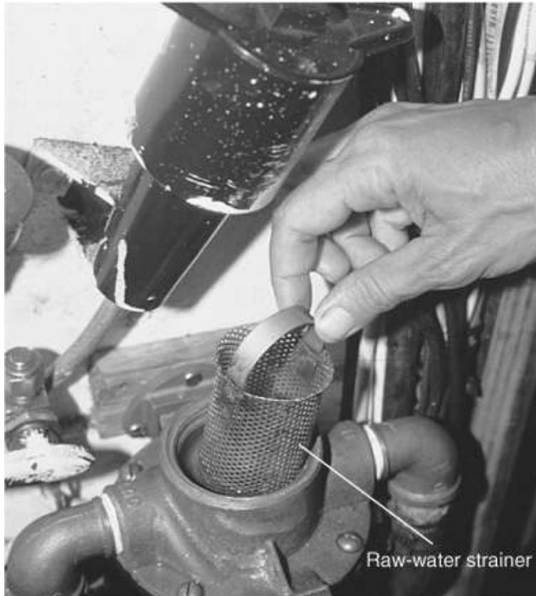
FIGURE 3-28. Removing the raw-water strainer for cleaning.
