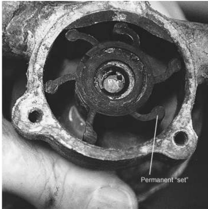
FIGURE 5-9. Even though the impeller tips are still curved, if the vanes retain a “set” after removal, the impeller needs replacing.
