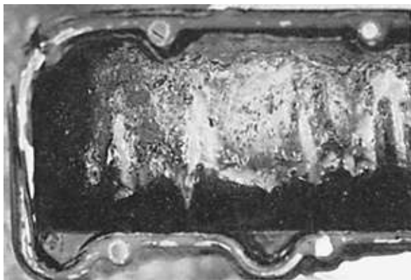
FIGURE 5-28. Emulsified oil inside a valve cover (the cover has been removed from the engine). In this instance, the problem was caused by a blown head gasket.
