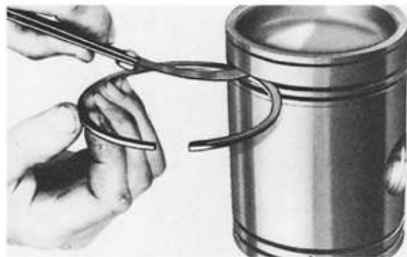
FIGURE 7-41. Measuring the vertical clearance between the ring and the groove. (Courtesy Caterpillar, top; Fritz Seegers, middle; Detroit Diesel, bottom)
