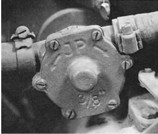
FIGURE 5-2. A typical raw-water pump.
