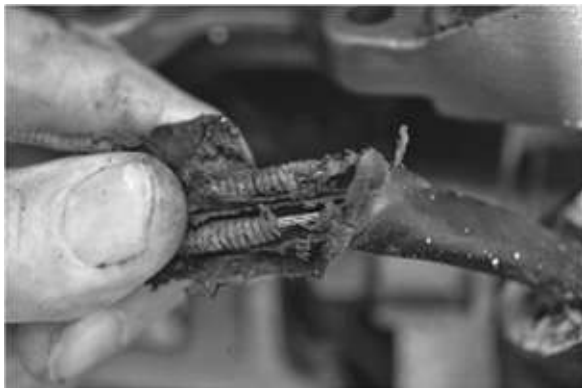
FIGURE 8-28. A corroded engine control jacket. The inner cable is stainless steel
