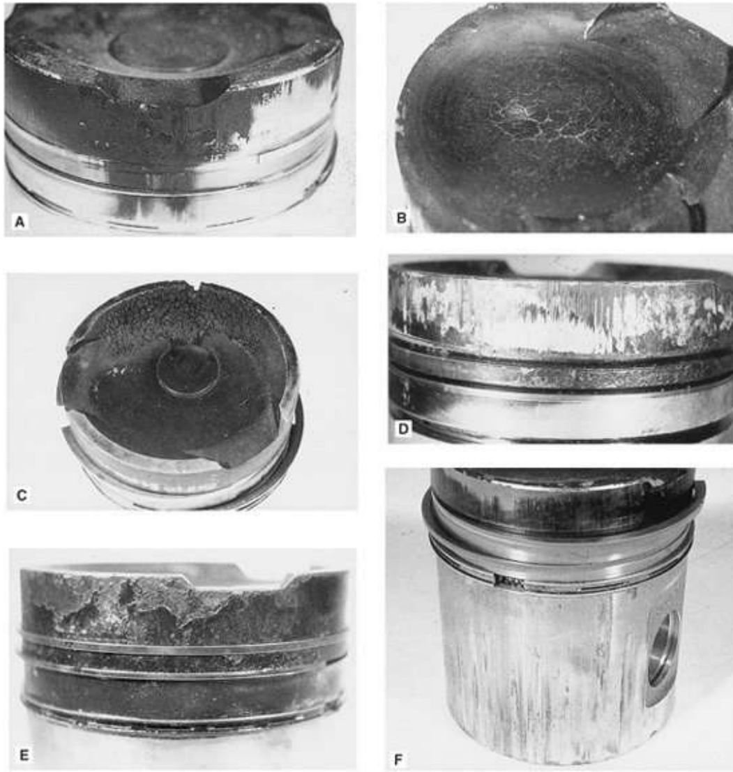
FIGURES 7-30A to 7-30G. Generalized overheating of the crown. The top of the piston side has started to peel away and stick to the cylinder wall (A); the piston cannot be used again. Cracking of the piston crown through overheating, in this case concentrated where the gases blow down out of the precombustion chamber (B); the piston cannot be used again. Severe erosion of the piston crown due to erratic combustion caused by a plugged air filter (C); this piston cannot be used again. The stainless steel plug in the crown, found only in high-performance engines, helps dissipate heat from the precombustion chamber. Carbon cutting around the piston top from the ring of carbon at the top of the cylinder (D); although the piston is scratched, it isn't breaking up and can be used after it has been cleaned. The rings on this piston are stuck in their grooves, leading to overheating, blowby, and serious erosion of the side of the piston (E); it cannot be used again. The skirt (the area below the piston pin) of this piston has been
