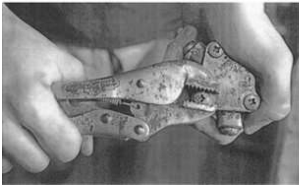
FIGURES E-3 and E-4. Using Vise-Grips to back out a stud and screw.
