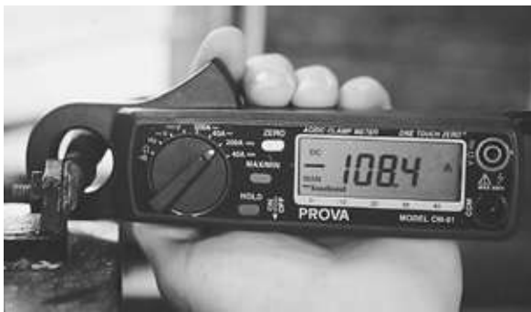
FIGURE 4-13. Testing the amp draw of a starter motor with a clamp-on DC ammeter.
