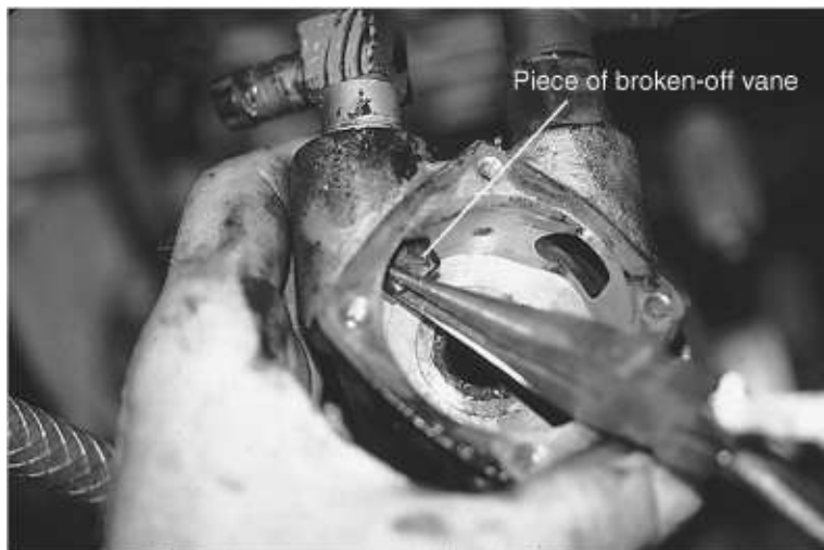
FIGURE 5-11. Tracking down the missing vanes from the impeller shown in Figure 5-3 . The first one was found in the pump discharge elbow; the second in the tubing; and the third...
