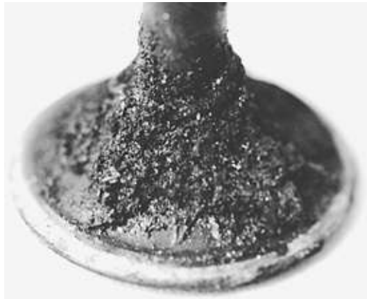
FIGURE 5-23. A heavily carbonized valve due to poor operating practices.
