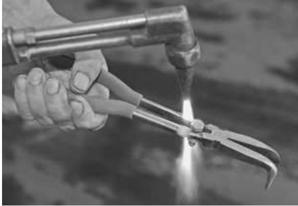
FIGURE 3-26. Heating the handles of a needle-nose pliers with an oxyacetylene torch.
