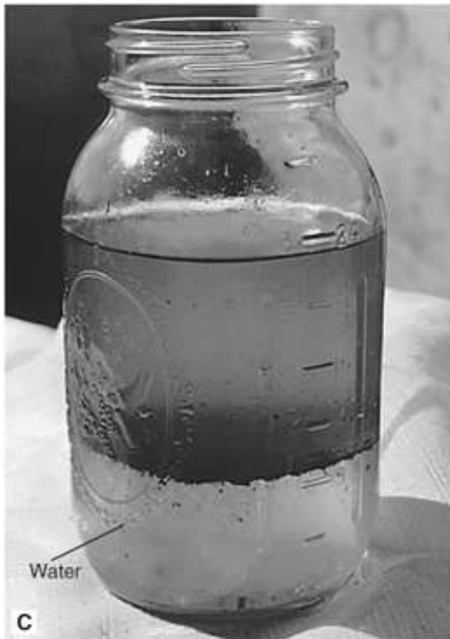
FIGURES 5-39A TO 5-39R. A do-it-yourself engine survey. Any kind of an engine log (in this case, written in the back of the engine manual) is important (A). Regular oil sampling is an excellent indication of attention to maintenance issues (B). Fuel tank sample showing significant water contamination. If any of this has made its way through to the injectors, there may be serious damage (C). An oil sample after 50 hours on a new engine; note that it is almost translucent (D). The same engine after 150 hours—the oil is black from carbon in suspension (E). This is normal, but any kind of sludge is a sign of trouble. Checking for sludge and emulsified oil inside the oil fill opening (F). Note the oil immediately beneath this water pump, coming from a leaking oil seal where the pump bolts up to the engine (this is a gear-driven pump rather than belt driven), and the salt crystals lower down from a leaking water seal (G). A rebuild is needed. Cracked
