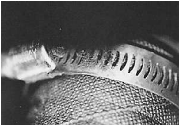
FIGURE 3-35. A perfectly good-looking “all-stainless” hose clamp, which, when the screw was backed off a turn or two, revealed considerable corrosion inside the screw housing, caused by using an inferior grade of stainless steel for the screw.
