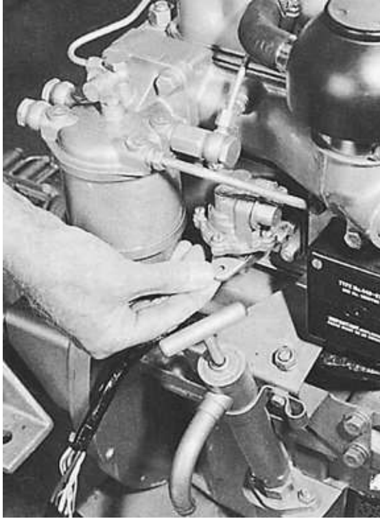
FIGURE 4-38. Operating a manual fuel lift (feed) pump. (Courtesy Perkins Engines Ltd.)
