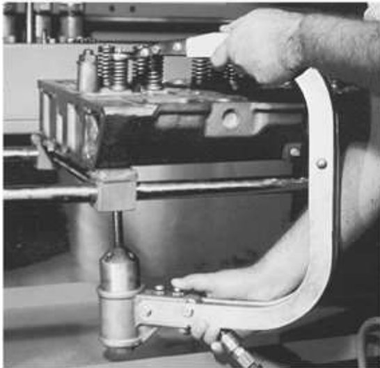
FIGURE 7-16. Top: Using a valve-spring compressor. (This is slightly different from the one described in the text, but it serves the same purpose.) (Courtesy Perkins Engines Ltd.) Bottom: A hydraulically operated valve-spring compressor in a large machine shop. (Courtesy Caterpillar)
