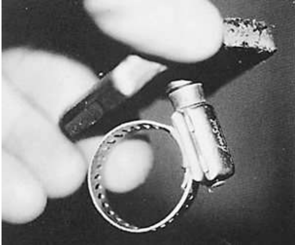
FIGURE 3-34. An “all-stainless” hose clamp with a screw of an inferior (magnetic), corrosion-prone grade of stainless.
