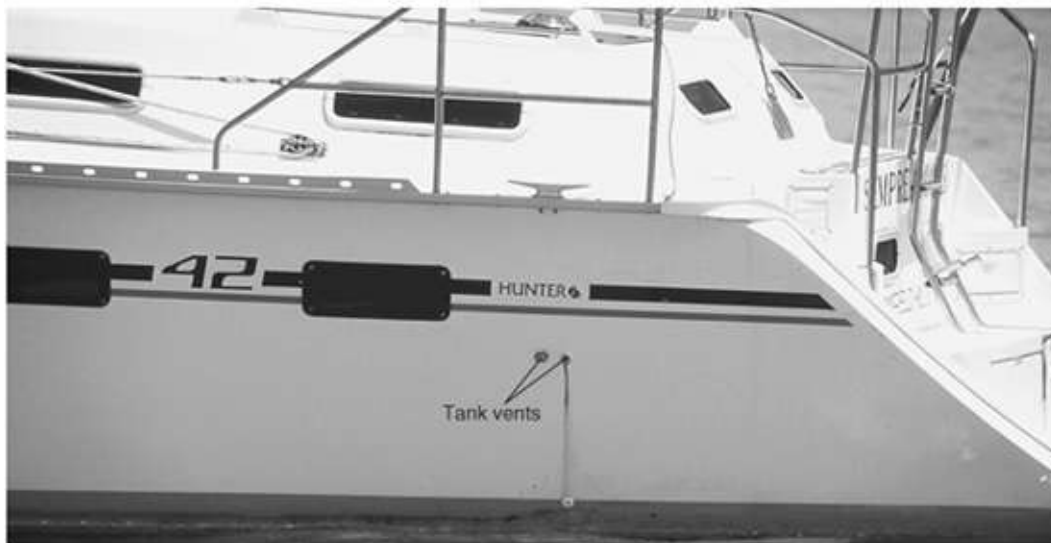
FIGURE 3-5. Tank vents in the side of a hull are an open invitation for saltwater contamination of the tank at some point.
