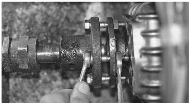
FIGURES 9-19 and 9-20. In this case, an appropriately sized socket is being used as a spacer to remove a stubborn coupling.
