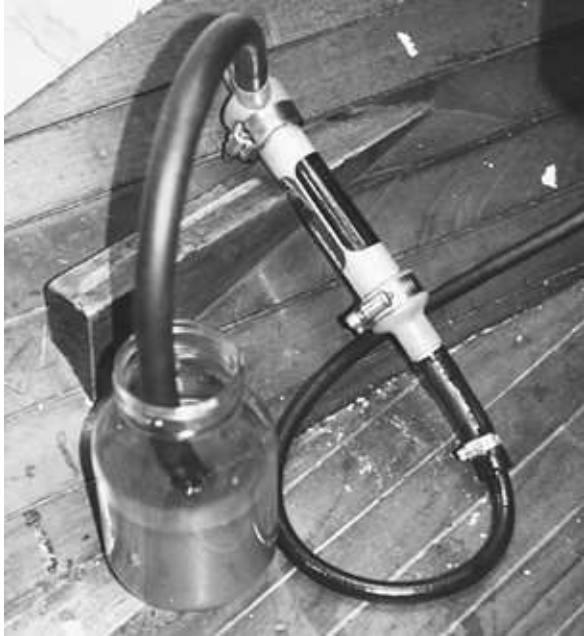
FIGURE 3-7. Pumping a fuel sample from the base of a tank.
