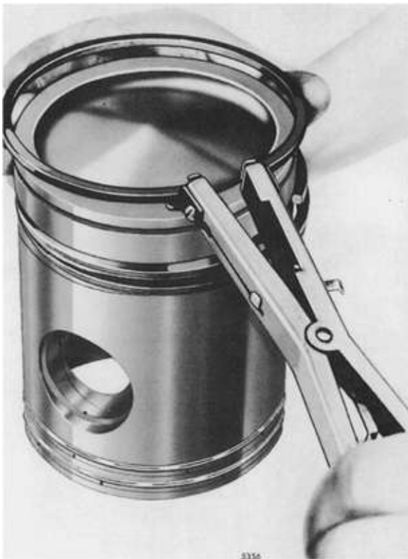
FIGURE 7-37. A piston-ring expander. (Courtesy Detroit Diesel)
