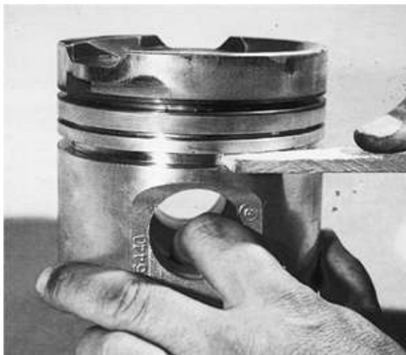
FIGURE 7-39. Cleaning piston-ring grooves with a piece of hardwood. (Courtesy Caterpillar)
