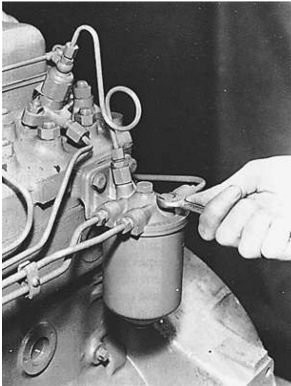
FIGURE 4-41.. Bleeding a secondary fuel filter. (Courtesy Perkins Engines Ltd.)
