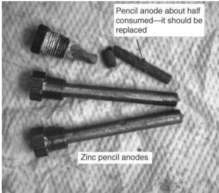
FIGURE 3-31. Many heat exchangers have zinc pencil anodes. These should be replaced when they are no more than half consumed.
