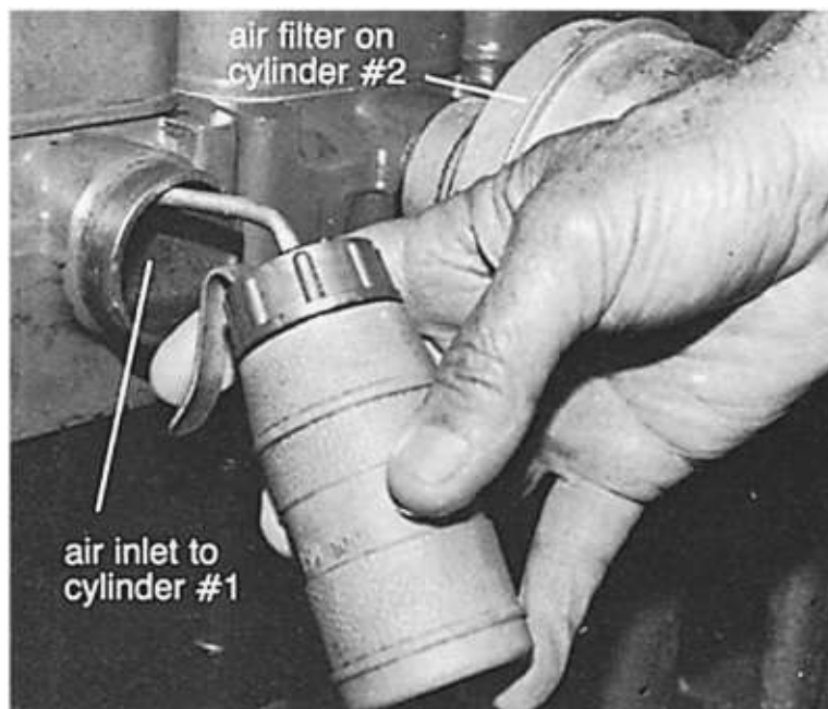
FIGURE 4-28. Adding oil to the inlet manifold to increase combustion chamber pressure.
