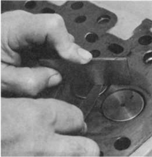
FIGURE 7-23. Checking for overgrinding of the valves. (Courtesy Perkins Engines Ltd.)
