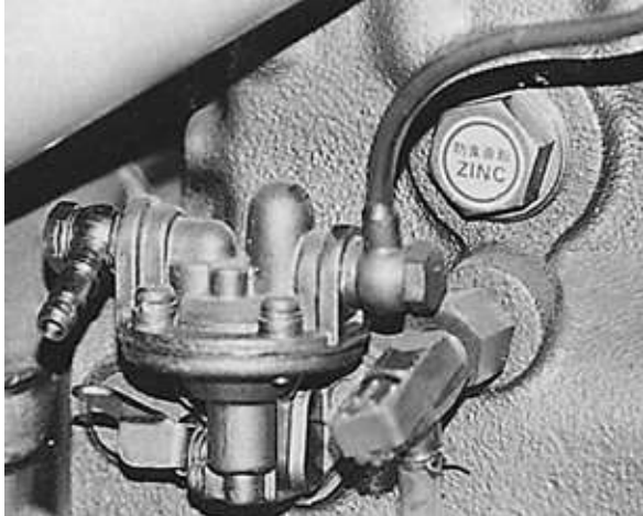
FIGURE 2-21. A typical mechanical lift pump fitted to the side of an engine block.
