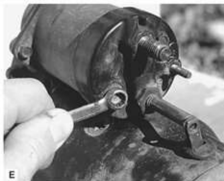
FIGURES 4-14A to 4-14K. Disassembling a preengaged starter's solenoid. First, identify the main components (A). Remove the battery cable (B). Disconnect the solenoid from the starter motor (C). Disconnect the cable to the ignition switch (D). Take the cover bolts off the solenoid (E and F). Bend the starter motor strap out of the way so the solenoid cover can be pulled off (G). Remove the solenoid cover (H); there is a spring in here that may fall out. A view of the contactor plate, showing the burned contactor (I). Note the severe pitting on the surfaces of the contactor (the circular disc) and the points (J). Sometimes the contactor can be flipped over to reveal an unused surface, and as in this case, the points can be rotated in their housing to bring a new surface into action (K). Otherwise, they can be filed and sanded smooth.
