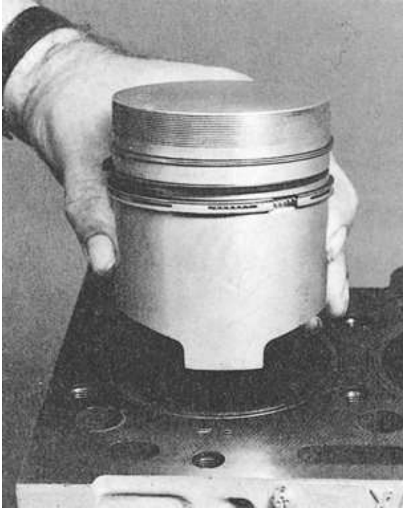
FIGURE 7-42. Lowering a piston into the cylinder. (Courtesy Perkins Engines Ltd.)
