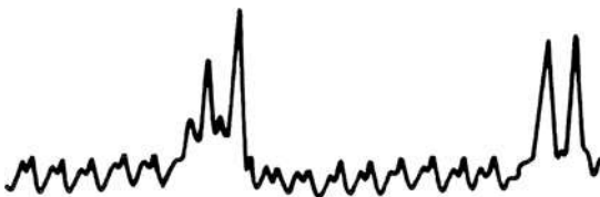
Figure 23.7 Typical hull pressure fluctuation indicating possible presence of PHV cavitation
