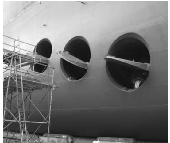
Figure 14.13 Doors fitted to a set transverse propulsion unit openings
