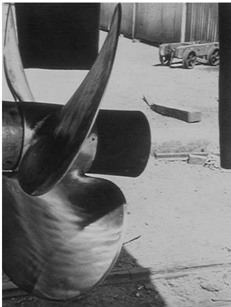
Figure 22.19 Truncated fairwater cone fitted to a high-speed patrol vessel
