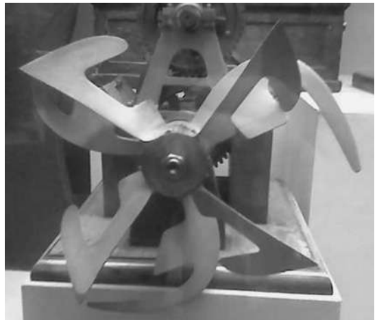
Figure 1.11 de Bay's contra-rotating propeller design
