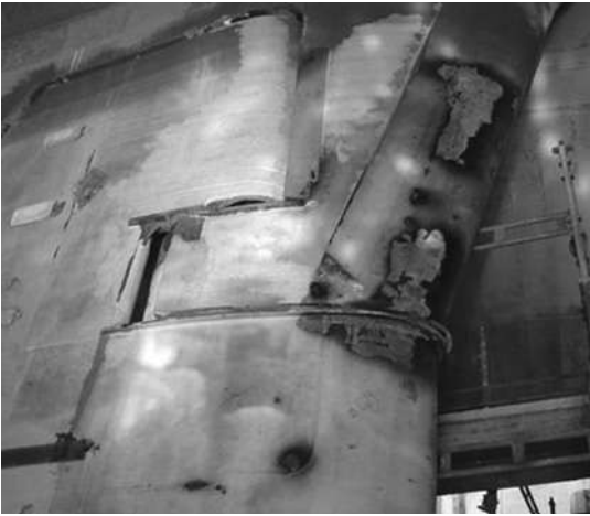
Figure 9.39 Example of rudder erosion
