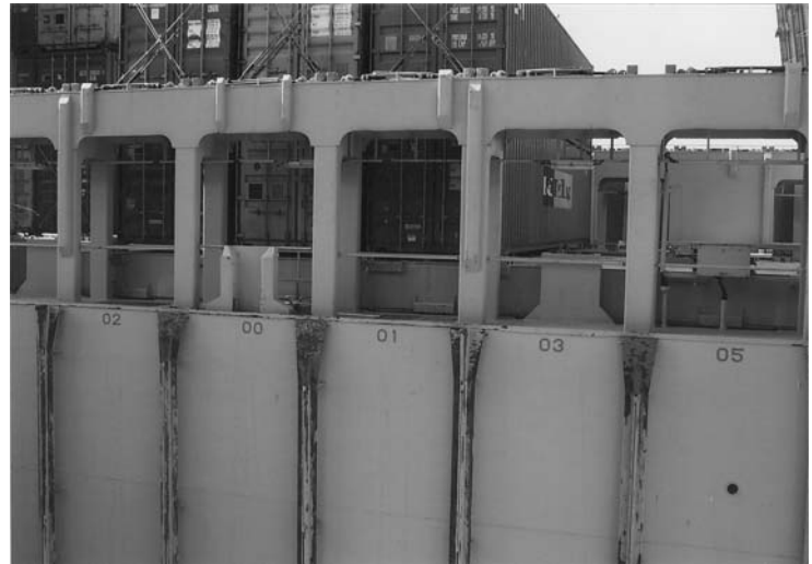
Plate 43. Cell guides exposed during the loading process of a container vessel. Containers above deck seen lashed in the stowed position.
