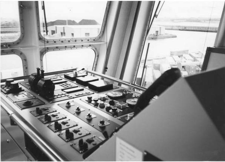
Plate 127. Bridge wing control station (enclosed) for a twin CPP, and bow thrust equipped aboard a modern Ropax Ferry.
