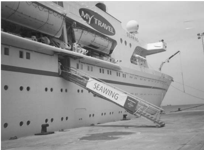
Plate 84. Department of Trade gangway, rigged at right-angles to the fore and aft line, with gangway net rigged, aboard the passenger liner 'Seawing' deployed from shell door. Angle from the horizontal should not exceed 30^{\circ} .
