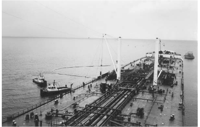
Plate 152. An oil tanker approaches a Single Buoy Mooring and has the midships. Port derrick deployed to recover the floating hose.
