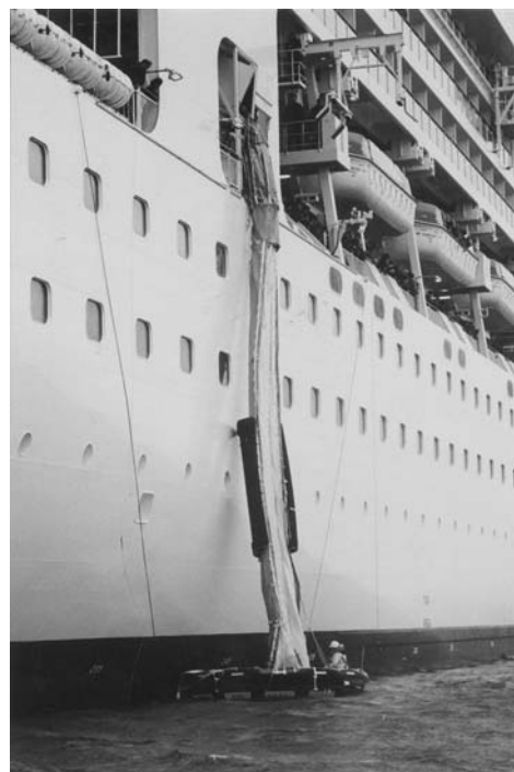
Plate 70. Single chute shown deployed with the surface landing platform. Life rafts are stowed aft of the MEC position.
