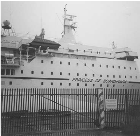
Plate 74. Rescue boat positioned abaft the navigation bridge starboard side of the passenger ferry 'Princess of Scandinavia'.
