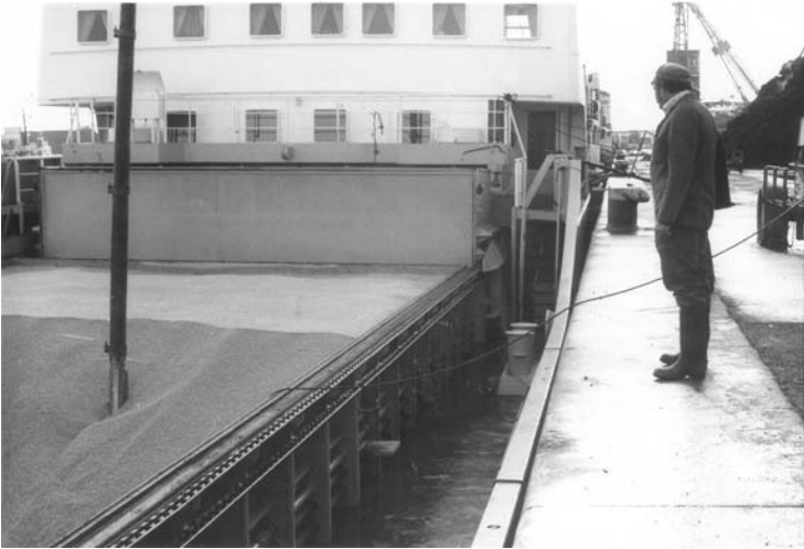
Plate 35. Open hatchway with steel covers stowed and secured at the aft end of the hatch. Grain suckers are engaged in discharging a bulk grain cargo.
