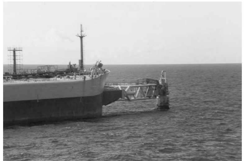
Plate 154. Oil riser and forward rigid arm connection to an on site FPSO.
