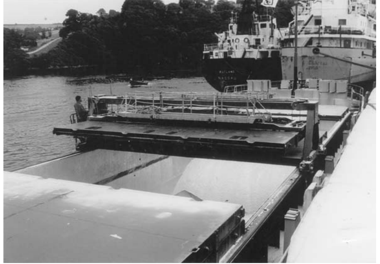
Plate 28. Stackable steel hatch covers aboard a modern coastal vessel. The ship is fitted with its own travelling mini gantry crane.
