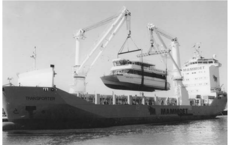
Plate 26. Heavy lift cranes work in tandem on project cargoes joint, remote control of both cranes is a general feature by the ships chief officer when working in this manner.
