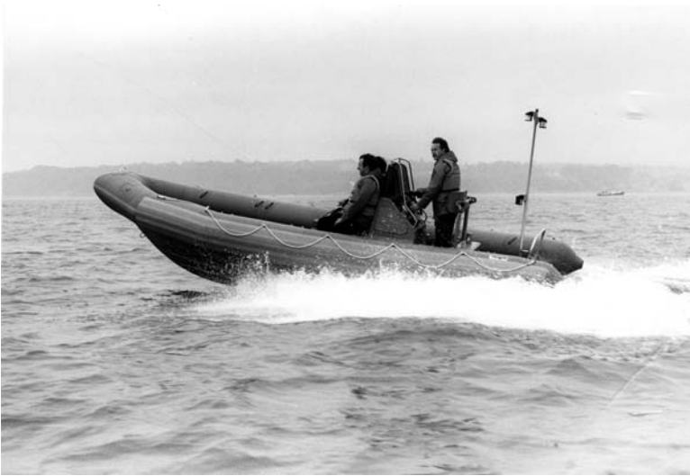
Plate 77. A 6.4m Avon Searider operating at speed is an example of a semi-rigid, fast rescue boat (FRC) now carried by many vessels.
