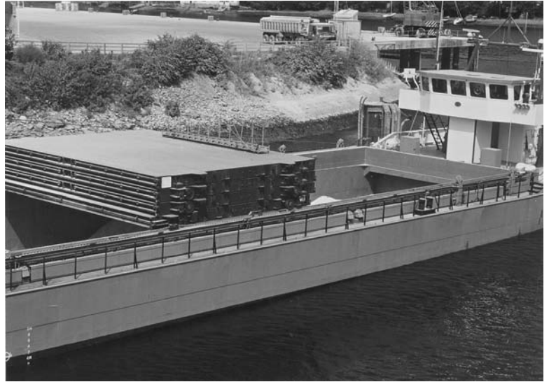
Plate 33. Horizontal, stackable steel hatch covers. The ship is equipped with its own mini track operated 'Gantry Hoist' designated solely for lifting, transporting and stacking of the covers (Gantry not shown).
