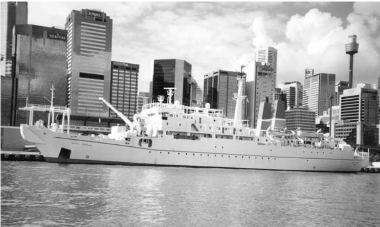
Plate 2. The cable vessel 'Pacific Guardian' lies Starboard side to the berth. The type of ship is distinctive with cable fittings at the bow and the stern positions.
