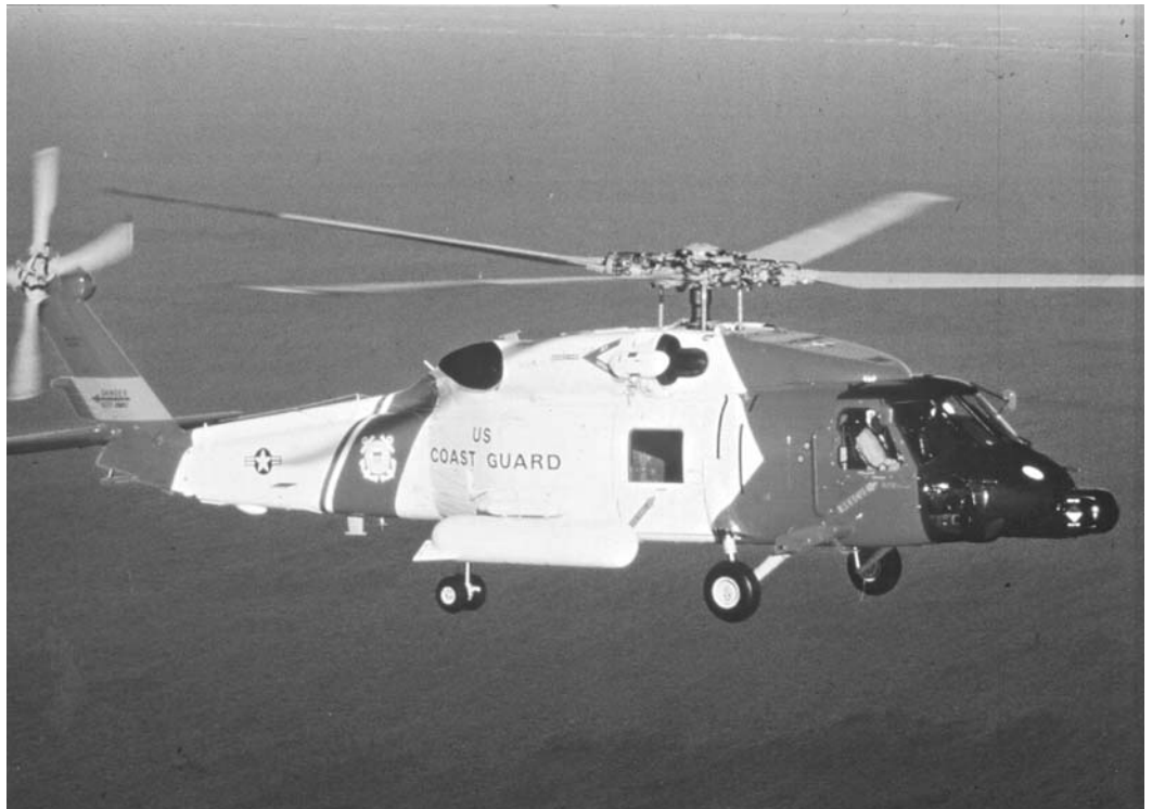
Plate 122. Sikorsky HH-60J Jayhawk operated by the US Coastguard, medium range recovery aircraft. Payload up to 8 survivors with 45 minutes endurance on scene.
