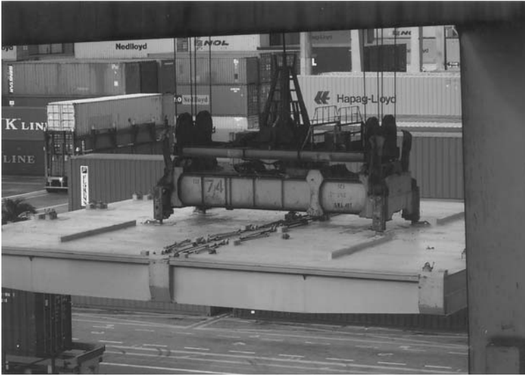
Plate 46. The container hoist engaged in lifting the pontoon hatch covers clear of the cellular holds.
