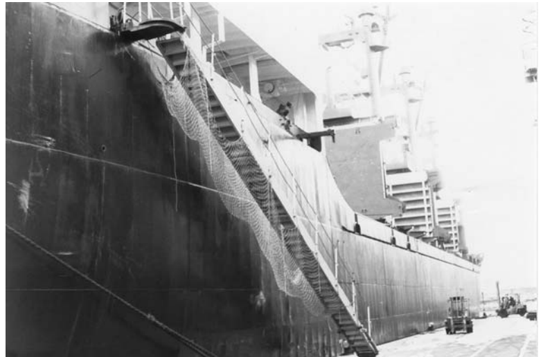
Plate 86. Accommodation ladder seen rigged with stanchions, manropes and gangway net landed to the quay with the bottom roller clear of obstructions.
