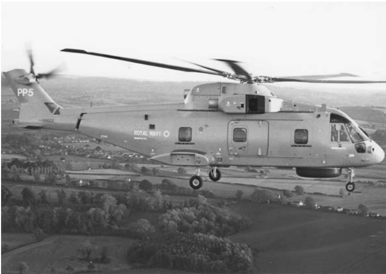
Plate 124. The latest rotary wing aircraft assigned to British Military Forces a triple engine, 5 Blade Rotor, 'Merlin.' Helicopter in operation with the royal navy.
