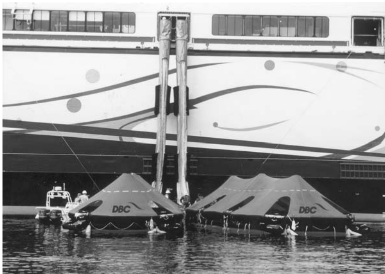
Plate 69. Double chutes deployed with life rafts at the waterline. Example configuration of MEC system as manufactured and produced by Dunlop/Beaufort – Canada.
