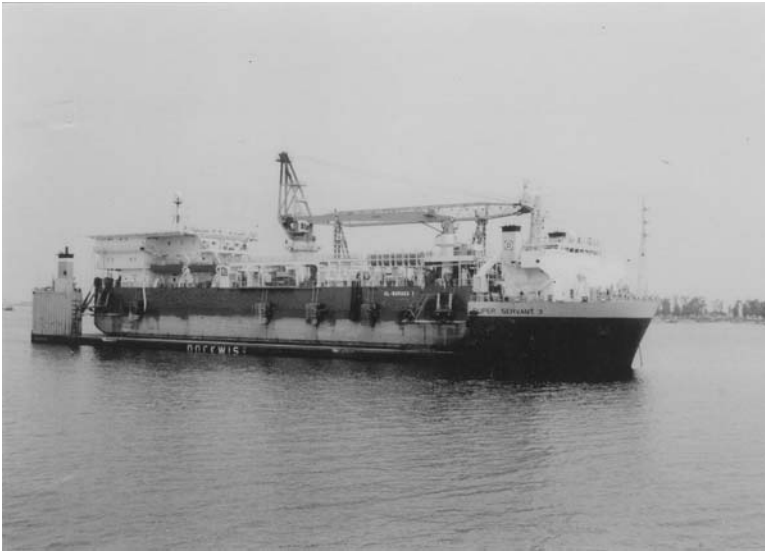
Plate 24. The heavy lift vessel 'Super Servant 3' engages in project cargo operations by transporting the offshore barge 'Al-Baraka 1'
