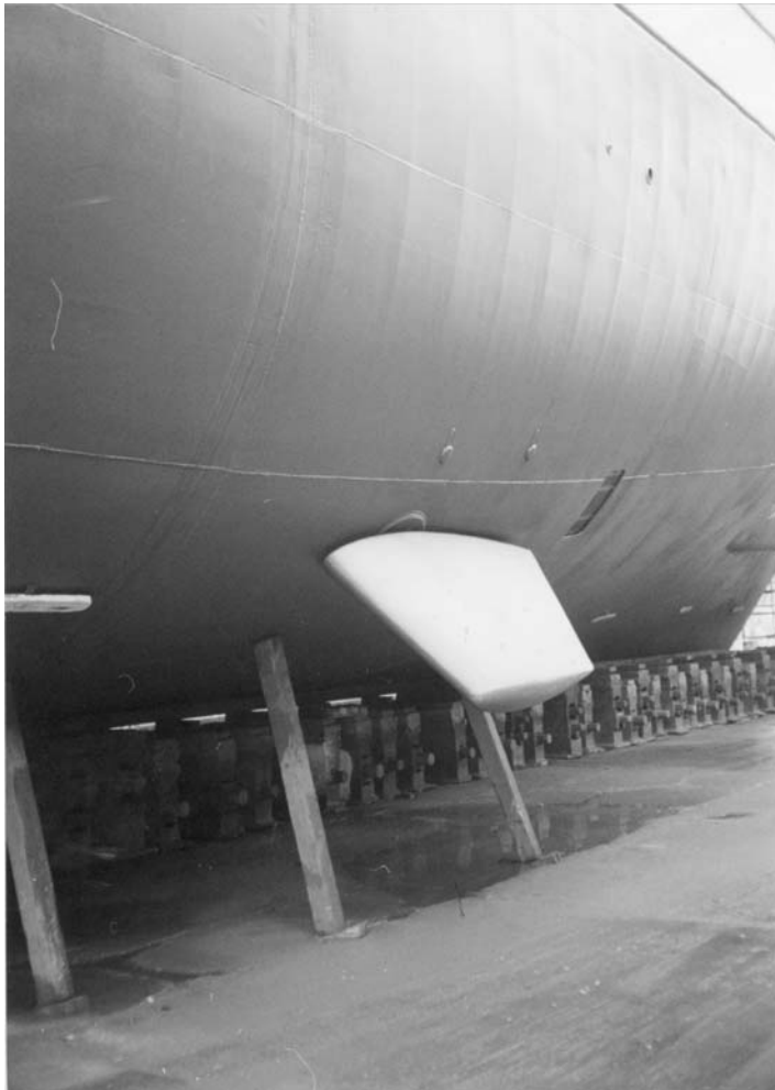
Plate 134. Fixed (Non-Retractable) stabiliser fin. Seen exposed on a vessel in dry dock.
