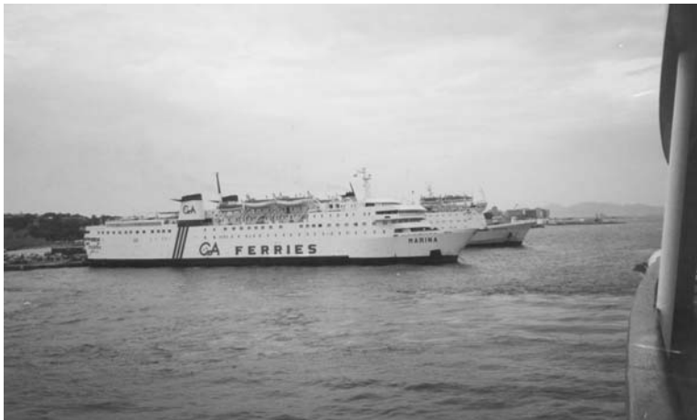
Plate 142. Passenger/vehicle ferries lie stern to the quay in Mediterranean moors in the Greek Island of Rhodes.
