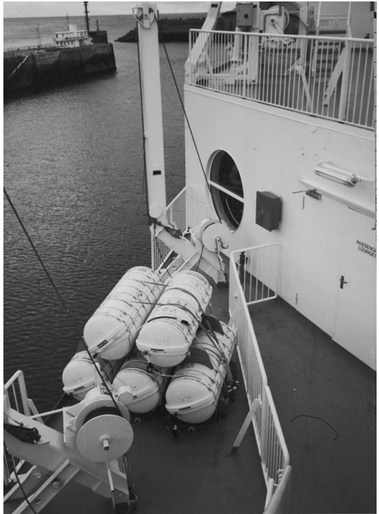
Plate 63(a). Rack stowage of inflatable life rafts aboard a passenger vehicle ferry.
