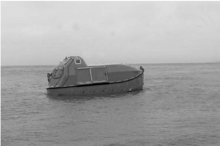
Plate 54. Totally enclosed lifeboat seen in the battened down situation at sea.
