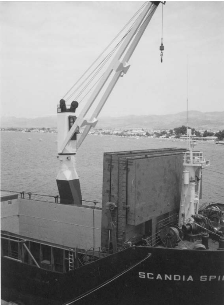
Plate 36. Hydraulic, vertical stowing steel hatch covers. Seen in the open position and secured back at the forward end of the open hatchway, aboard the 'Scandia Spirit' dry cargo vessel. One of the two 35 tonne, SWL cranes is sited in the background on the Port, offshore side.
