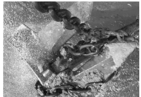
Plate 16. An AC14 anchor shown fouled on its own cable.
