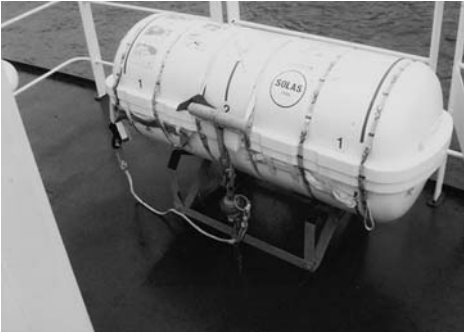
Plate 66. Inflatable life raft stowed in cradle and fitted with hydrostatic release unit.
