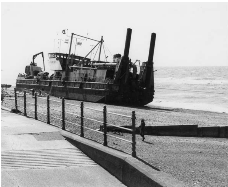
Plate 111. A flat bottom dredger blown aground, side on to a sand and gravel beach in bad weather off the north west coast of the UK.
