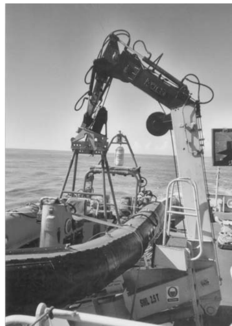
Plate 76. Single arm launching system for semi-rigid fast rescue craft operates up to 2.5 tons SWL the boat is gripped in, by quick release web straps and provided by a crew boarding platform.
