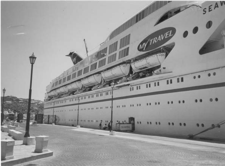
Plate 56. Open lifeboats stowed on the starboard side of the passenger cruise liner Seawing.
