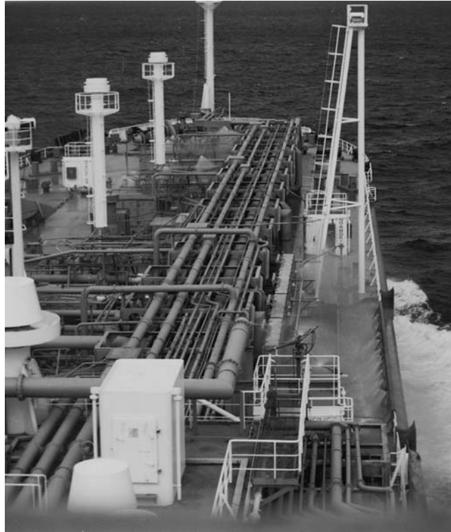
Plate 48. Fore end view of tanker vessel at sea pipeline and ventilation arrangements illustrated.
