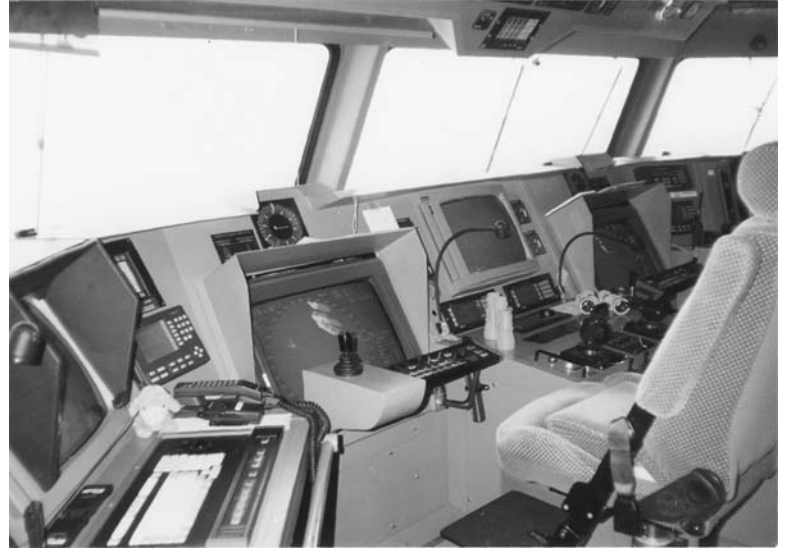
Plate 80. Example bridge layout as seen looking forward through the bridge windows from the auto pilot/steering position. Multi functional ARPA and communication consol set either side of centre.
