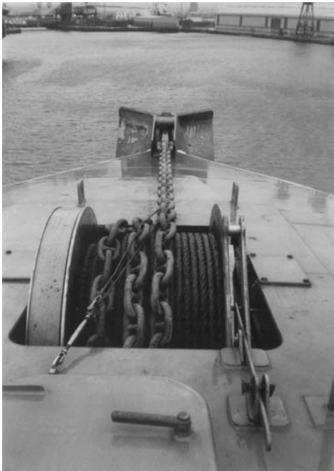
Plate 15. Single centre line anchor arrangement in the bow of a high speed craft (HSC) ferry use of combination chain cable and anchor warp.
