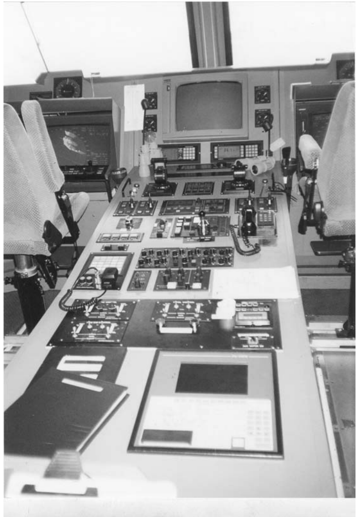
Plate 126. Central bridge control consol set into the integrated navigation bridge of a modern high speed craft.
