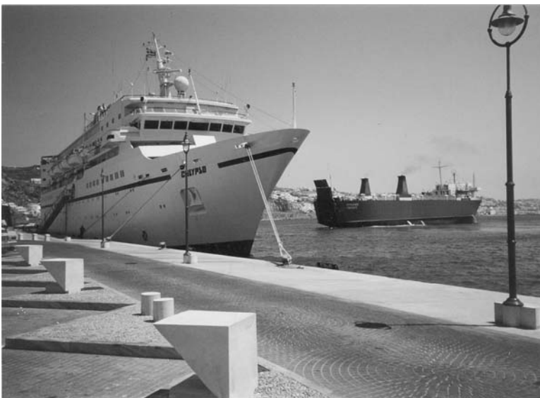
Plate 138. The 'Calypso' Passenger cruise vessel lies starboard side to, moored by head lines and rope springs while the Ro-Ro vehicle ferry 'MYKONOS' turns off the berth, to navigate stern first to the link span ramp.
