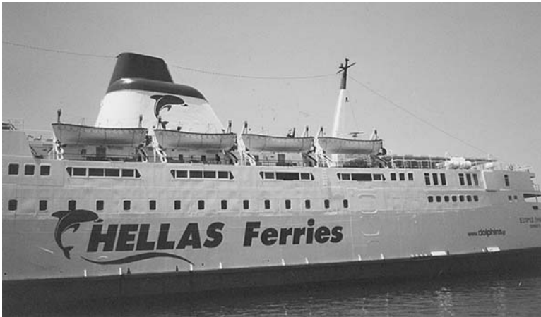
Plate 50. GRP open lifeboats stowed in gravity davits aboard the 'Express Penelope' a Ro-Ro passenger ferry & operating in mediterranean waters.
