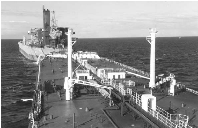
Plate 151. A pair of Samson posts and 5 ton S.W.L. derricks in a midships position on an oil tanker as it approaches a floating storage unit (FSU). Two smaller deck cranes are also sited aft of each Samson post. On this occasion the ship's lifting gear will not be employed as the ship will engage with forward moorings and the fore end manifold. The FSU being fitted with an oil pipeline bearing boom seen exposed at the aft end of the unit. Once the pick up mooring buoys have been recovered the tanker will pick up forward moorings and the 'boom' would be lowered to effect transfer.
