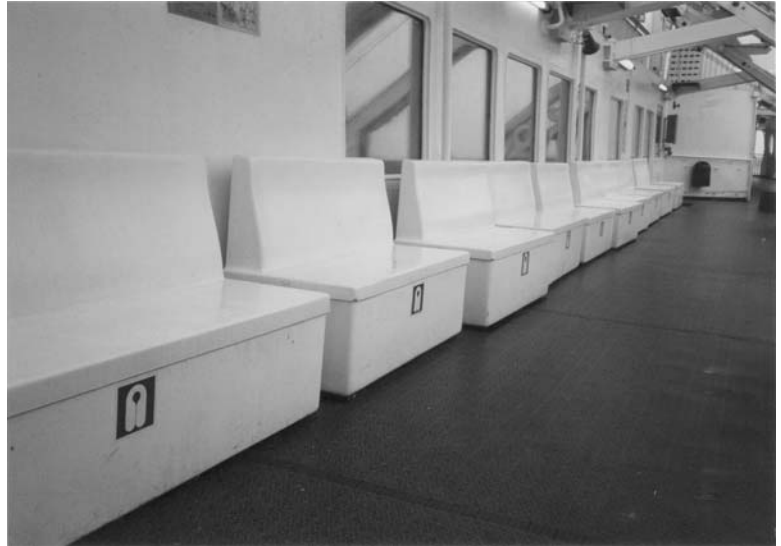
Plate 71. Life jacket stowage arrangement on the embarkation deck of a passenger ferry as fitted with overhead gravity davits.
