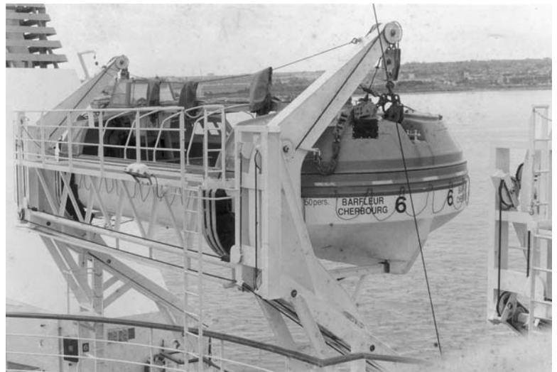
Plate 53. A 60 man partially enclosed lifeboat seen in the stowed position aboard the 'Barfleur' passenger/vehicle ferry.
