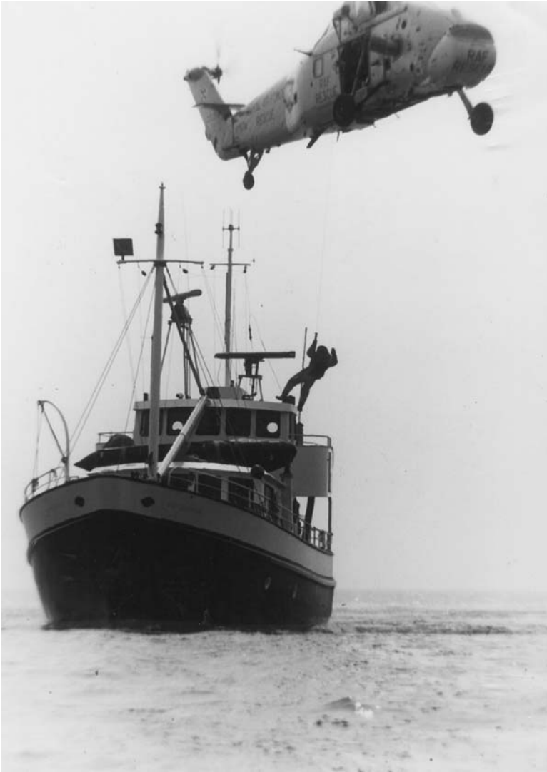
Plate 121. A Wessex MK4 SAR helicopter of the RAF lowers aircrew member to the deck of a motor fishing vessel.
