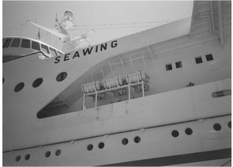
Plate 62. Racked inflatable life rafts stowed aboard 'The Seawing' cruise liner.
