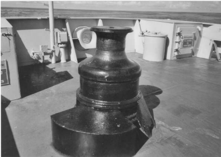
Plate 136. Single (Old Man) roller lead. Such examples can be motorised to work as a capstan.
