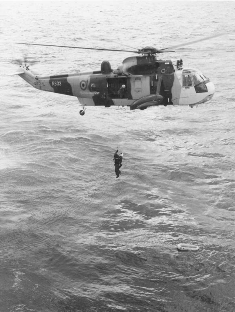
Plate 125. A Sea King helicopter from the Belgium military engages in an SAR operation making a single hoist from a survival craft.
