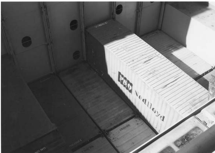
Plate 44. Twenty and forty foot container units stowed in the cell guides aboard a large container vessel.
