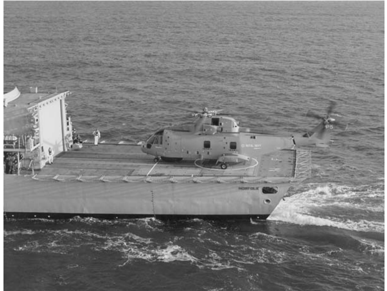
Plate 120. The 'Merlin' helicopter seen on the landing deck of 'HMS Norfolk' a type 23 frigate of the Royal Navy.
