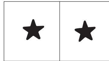
Figure 11.5 Images of true and reflected stars, showing side error.
