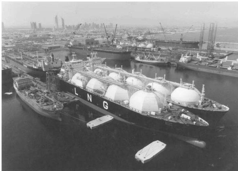
Plate 123. Two LNG carriers lie along side each other outside the Dubia shipyard. Prominent features being the gas dome structures on the upper decks.
