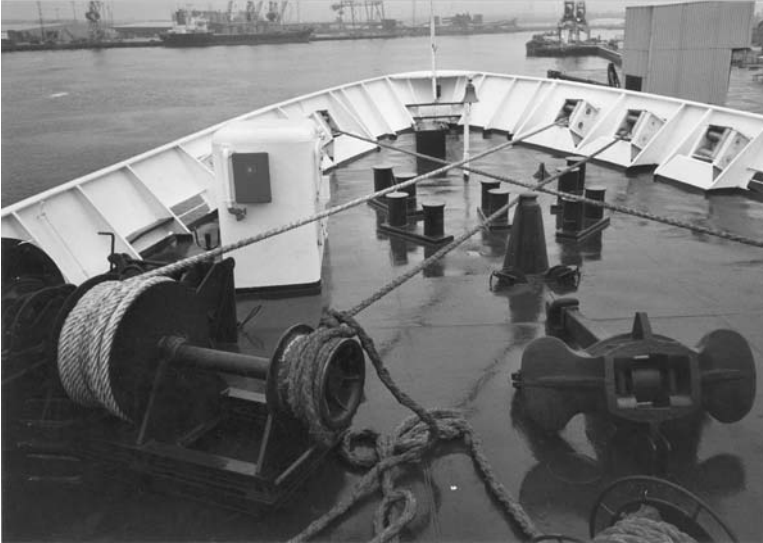
Plate 12. Fore deck of a Passenger vehicle ferry with split windlass arrangement incorporating a powered warping drum. An additional mooring is on the end rope drum.
