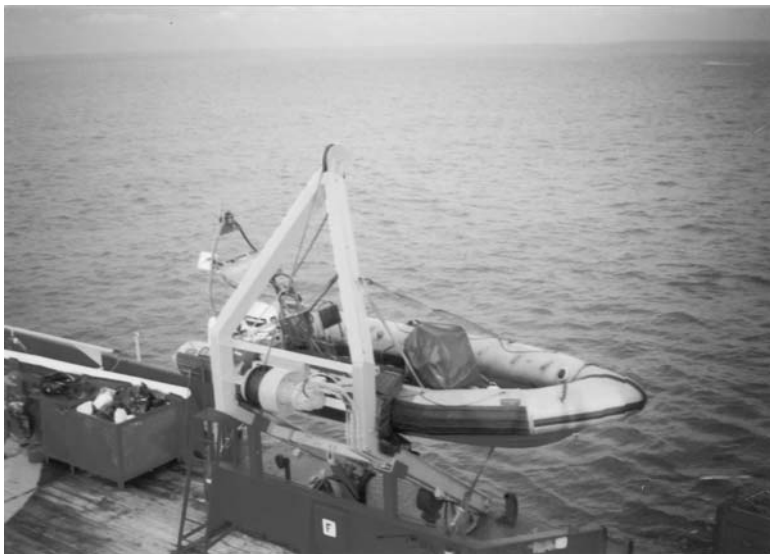
Plate 75. Typical offshore operation of an 'A' frame launching davit for operation with semi-rigid inflatable rescue boat.
