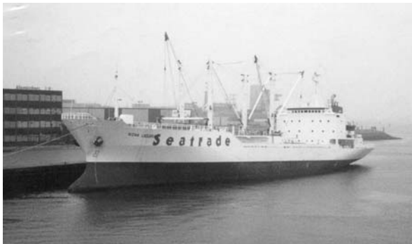
Plate 7. General cargo vessel 'Nova Liguria' lies alongside in the port of Amsterdam. Note all aft accommodation and derricks throughout, no cranes.
