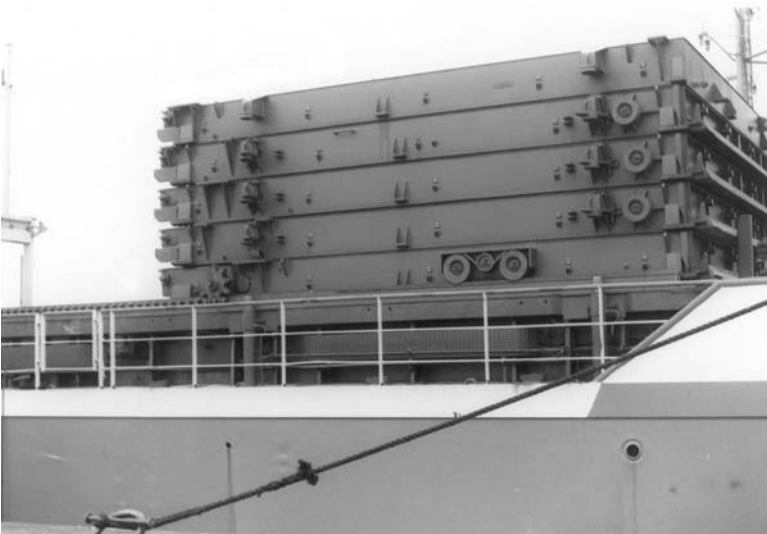
Plate 32. Rack and pinion horizontally stowed steel hatch covers.
