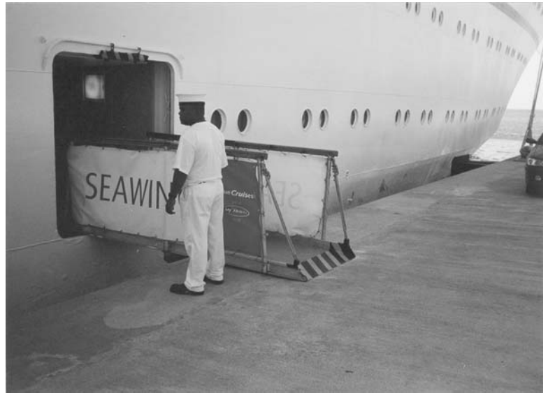
Plate 85. Alternative short gangway deployed from lower shell door from high freeboard vessels.
