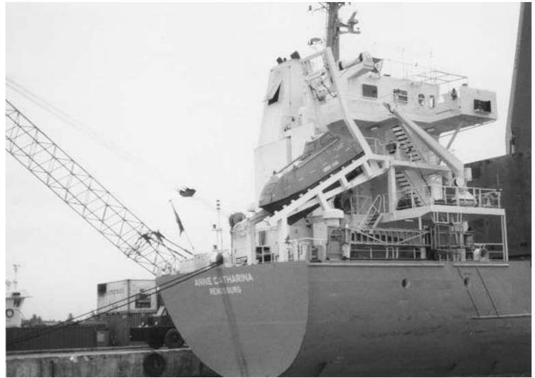
Plate 59. The general arrangement of the Free Fall Lifeboat over the stern of the 'Anne Catharina'. The davit launched liferaft is seen in an operating position over the starboard quarter.
