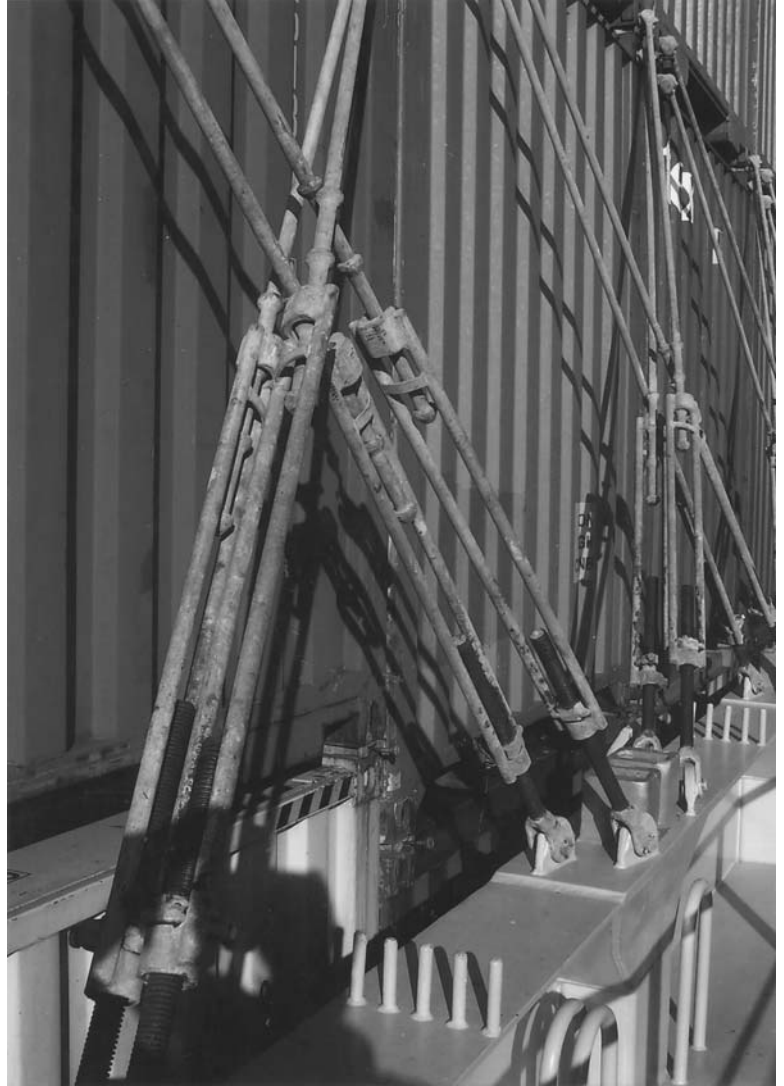
Plate 45. Container lashing bars, seen secured from the pontoon to the second tier of deck containers.
