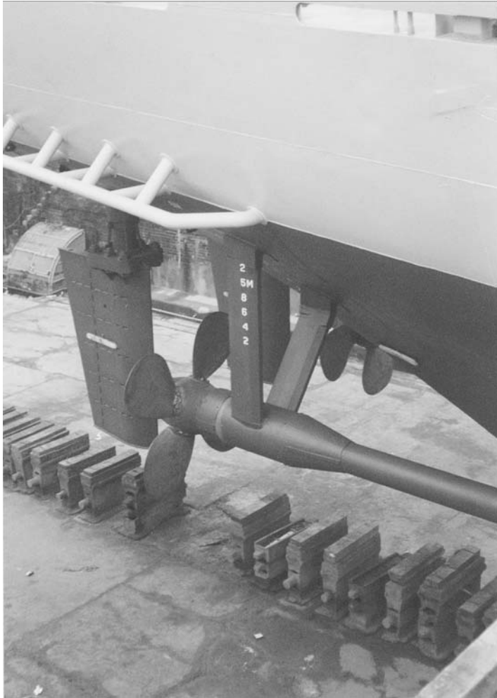
Plate 128. Structural support for twin screw/twin rudder vessel seen in dry dock where each tail end shaft is supported by struts extending from each quarter of the hull.
