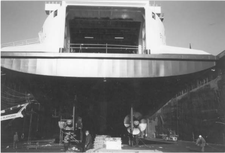
Plate 129. Modern ferry with twin screw (CPP) and twin rudder arrangement seen exposed in dry dock.
