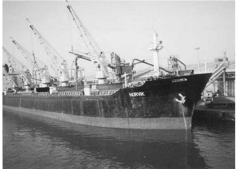
Plate 37. The general cargo vessel 'Norvik' with her deck cranes turned outboard to allow grain suckers to discharge bulk grain.
