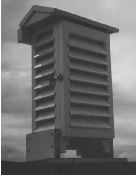
Plate 95. Stevenson's screen contains wet and dry bulb thermometers displayed in open aspect.
