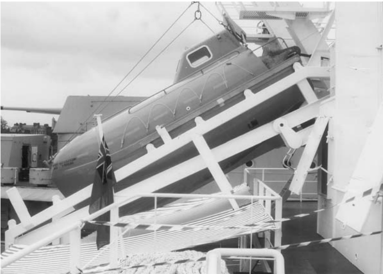
Plate 58. Free Fall Lifeboat seen being re-secured to the ramp in its stern launch position. The wire bridle is employed for recovery by the secondary means of launching, namely a davit/crane or derrick arrangement.
