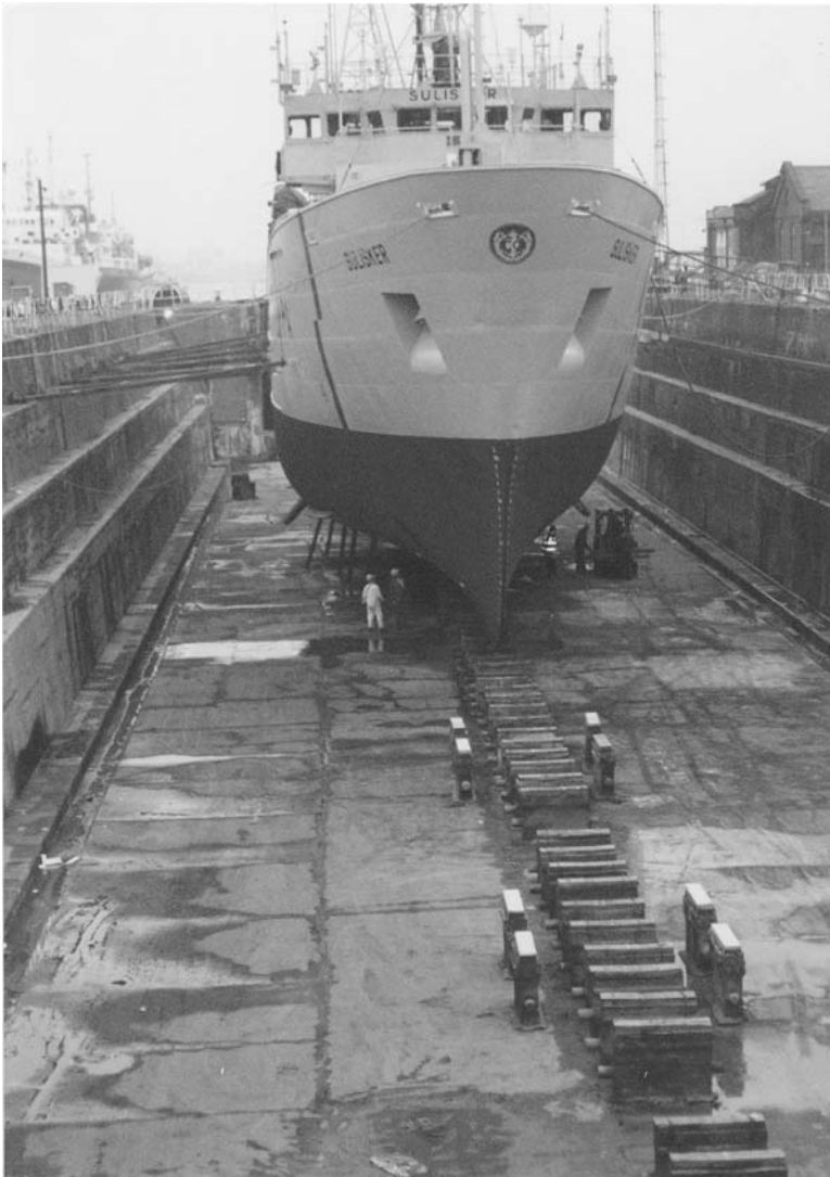
Plate 112. Dry Dock – Block Arrangements. The ‘Sulisker’ Sea Fishery Protection Vessel, lays on keel blocks in the William Wright, Graving Dock, in Hull, United Kingdom. The vessel is also supported at the sides by ‘wale shores’ and at the turn of the bilge with additional bilge chocks from the floor of the dock.
