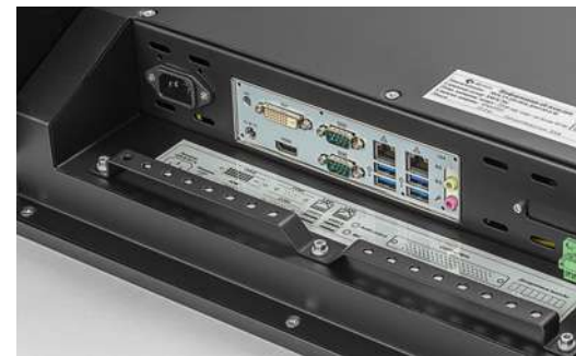
Panel with connectors for connection of MOS-19 marine computer equipment
