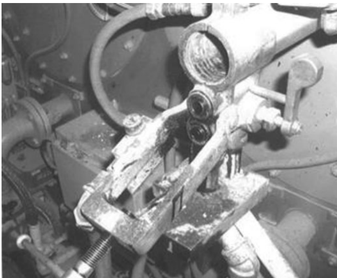
Figure 10-56. Yoke coupling clamp and set screw.
