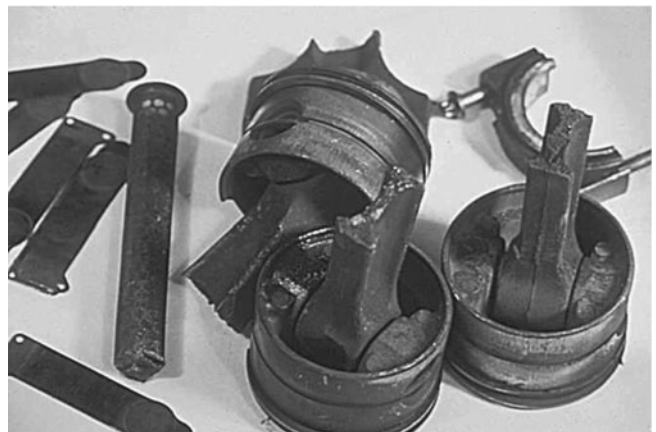
Figure 5-18. Broken compressor piston rods.
