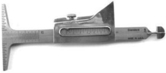
Figure 6-15(a). Welding inspection gauge.
