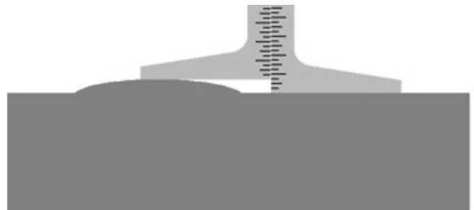
Figure 6-22. Check for excess external reinforcement.
