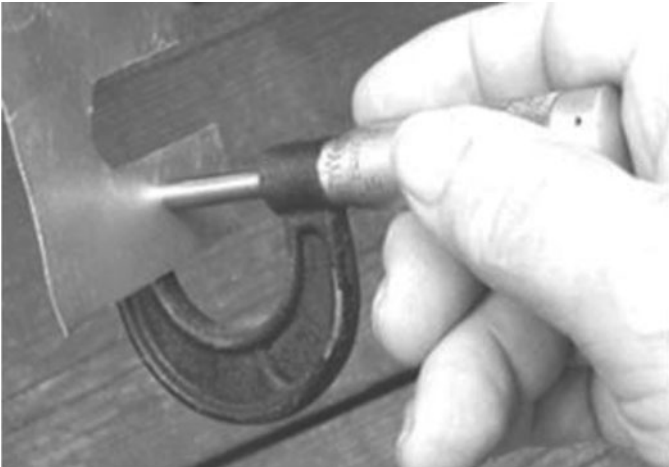
Figure 10-66. Measuring shim stock with micrometer.
