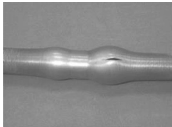
Figure 5-30. Chiller tube after freezing.
