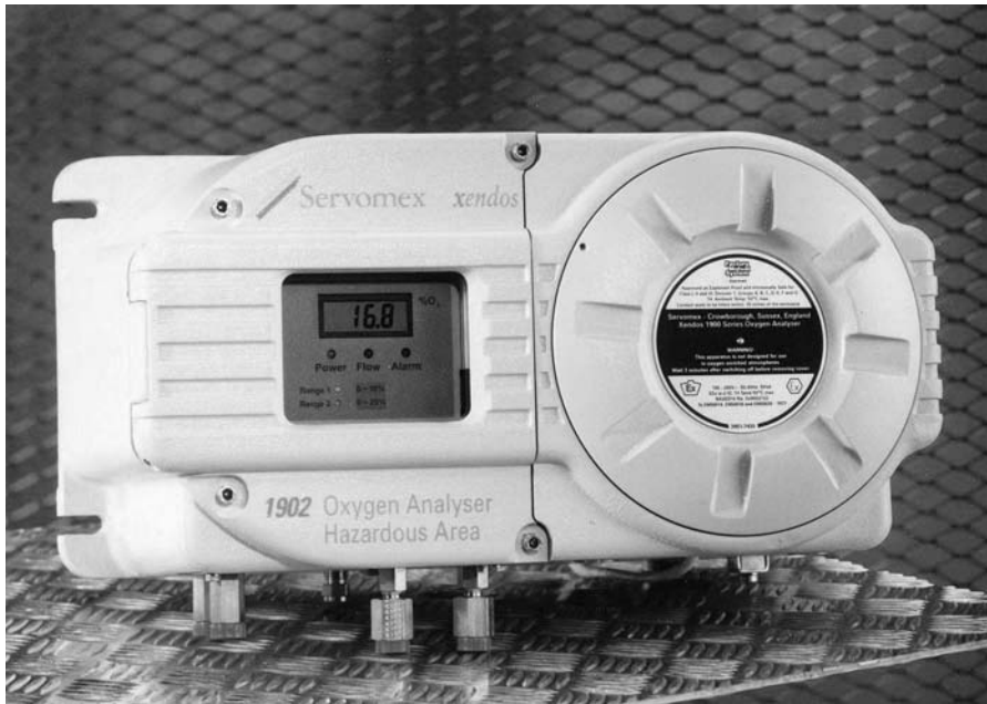
Figure 25.8 Example of a mixed concept apparatus which aids routine maintenance and adjustment. The circular threaded cover allows entry to a flameproof chamber and so must only be opened when de-energised, and under any other specific conditions which might be stated on the unit or in the associated documentation. The chamber behind the display contains only intrinsically safe circuits, thus permitting it to be opened at any time to allow access to, and live adjustment of, calibration or alarm setting controls, but subject of course to any extra operational conditions laid down by the manufacturer. Photograph courtesy of Servomex Group Ltd
