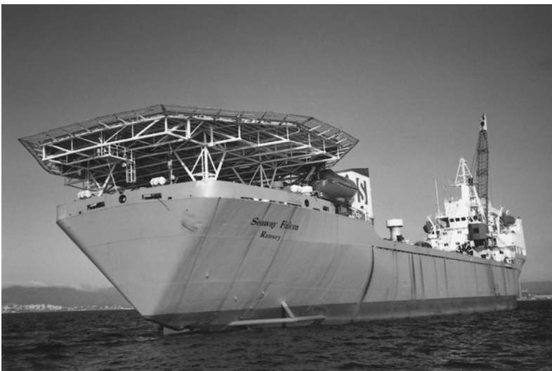
The 'Seaway Falcon' originally built as a drill ship, but later converted into a cable ship fitted with a dynamic positioning system.
