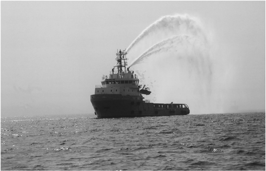
The 'Pacific Retriever', an anchor handling vessel, displays its powerful fire water monitors while on trials off the Coast of Korea.
