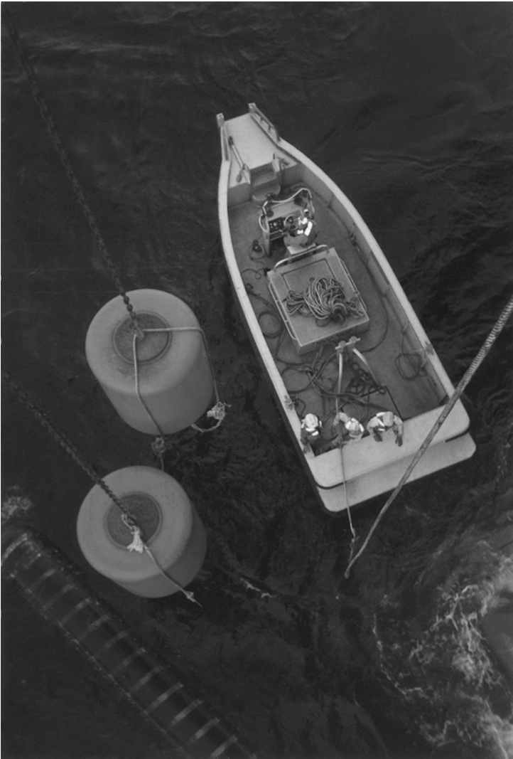
A mooring boat engaged in securing chain mooring recovery buoys for a shuttle tanker mooring to a Floating Storage Unit (FSU).
