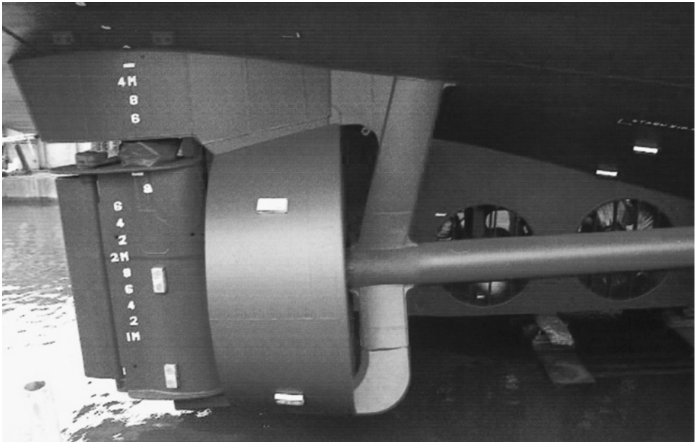
Stern arrangements with ducted propellers. Flap rudder aft of the propeller duct on a new build twin screw anchor handling vessel. Twin stern thrusters are seen built into an enhanced skeg. The whole area is fitted with sacrificial anodes because of the use of dissimilar metals employed in the manufacture of the hull and propeller units.
