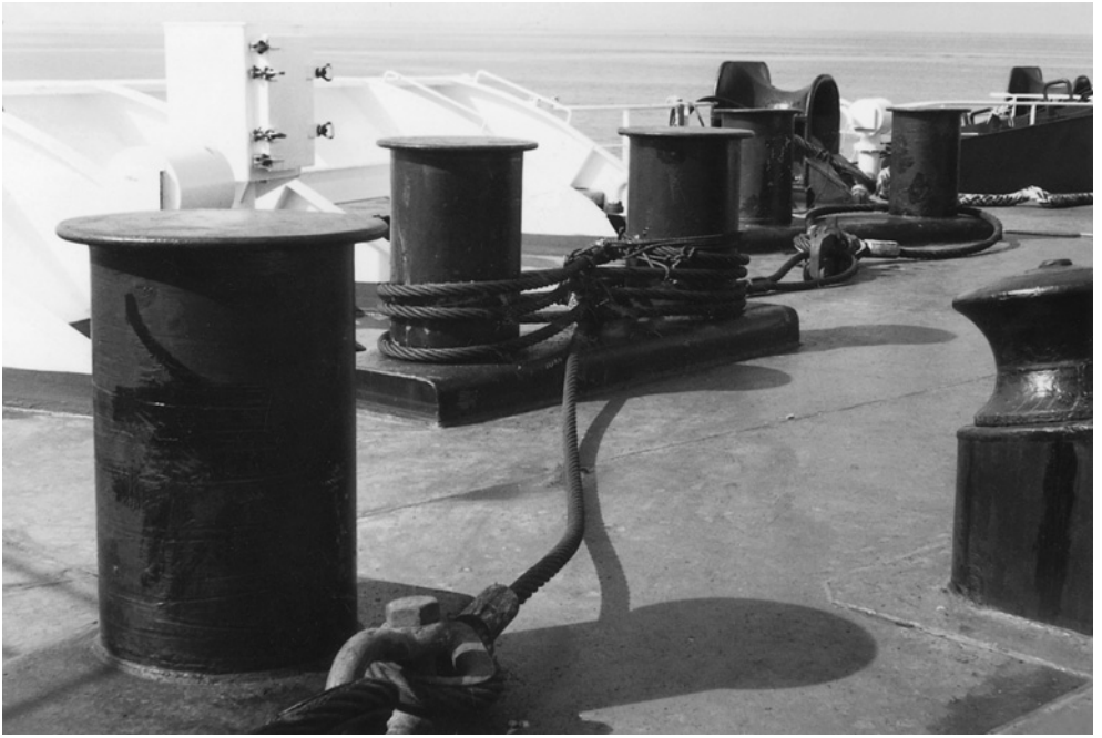
Double sets of bitts set on board the mooring deck of an offshore 'Anchor Handling' vessel. A stopper wire is seen being laid in 'Figure 8s' about the centre pair, the upper turns being lashed to prevent the wire springing off the 'Bitts' when under tension.
