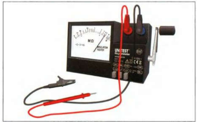
Figure 1.8a - Insulation resistance (IR) tester
