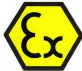
Figure 6.2 - European Ex identification mark
