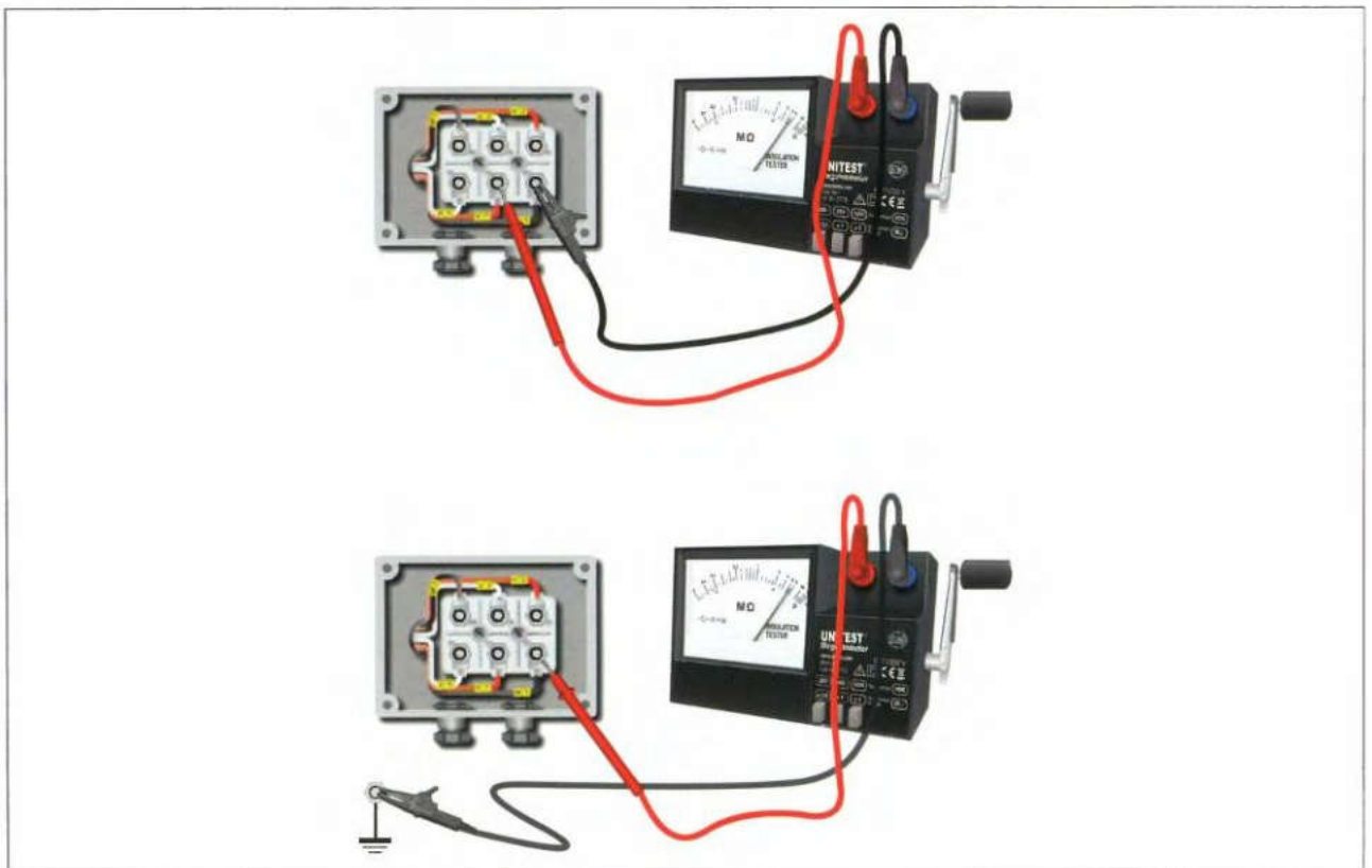
Figure 7.2 - Induction motor's insulation resistance (IR) test
