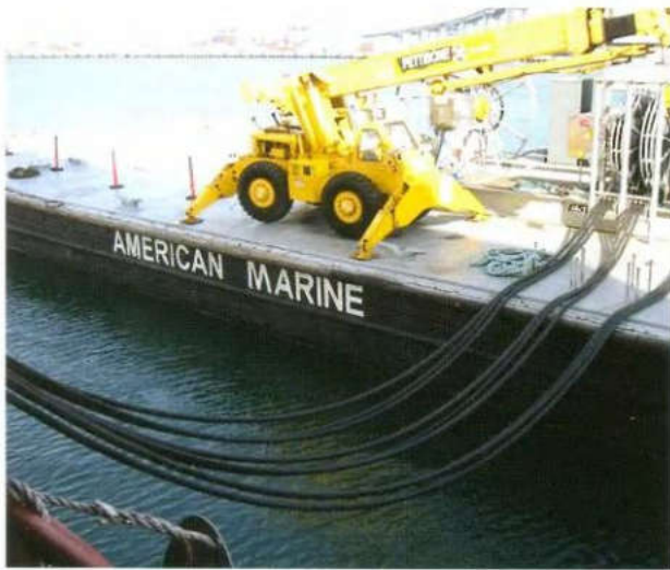
Figure 2.24 - AMP – barge mounted
